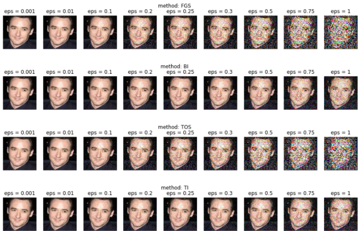
Figure 13: Adversarial samples for FGS, BI, TOS and TI as a function of perturbation norm
