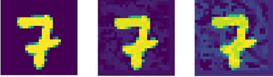
Figure 2.5: Left : Unperturbed image of a 7, Middle : perturbed image using the correct box constraint, Right : perturbed image without box constraint
