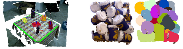
Figure 3: Examples of showing object segmentation results: (left) segmentation of isolated objects; (center) a pile of objects; (right) segmentation of the pile of objects.
