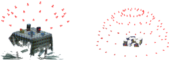
Figure 9: Accumulated view and camera pose: (left) Imperial College dataset; (right) generated synthetic dataset.
