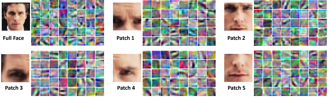
Fig. 4. Convolutional kernels computed. Each block corresponds to a selected patch with its learnt convolutional kernels in the first layer. Clearly, the learnt kernels are different for different facial patches.
