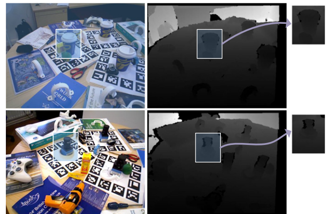
Fig. 4. Dataset generation: input of the proposed architecture is the depth image of a coarsely detected object (RGB correspondence is for better visualization).
